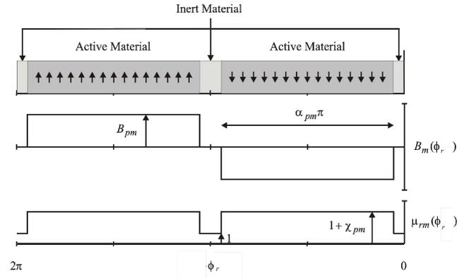
Fig. 4. Developed diagram of permanent magnet region.
