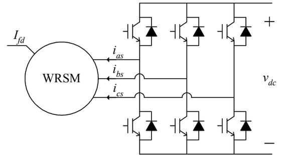
Fig. 6. System III. WRSM with active rectifier.
