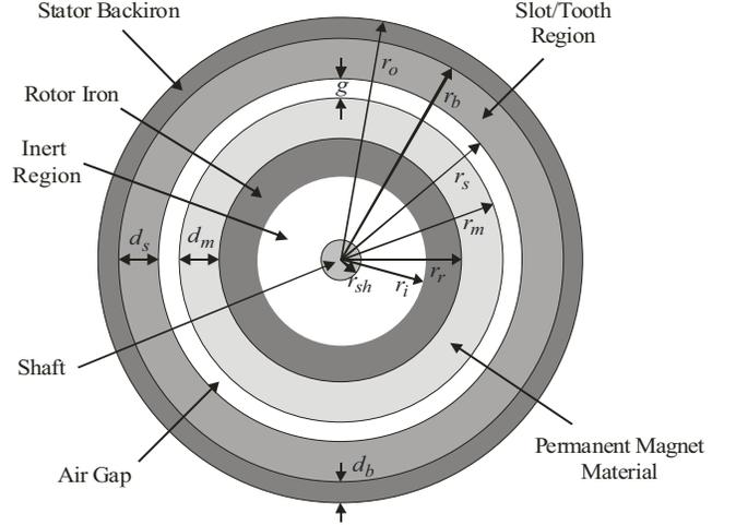
Fig. 3. PMSM Configuration.
